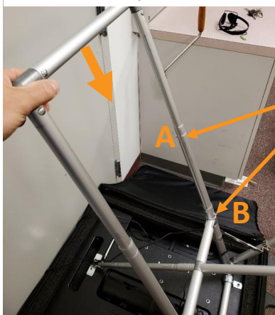
Figure 82. Collapsing Rear Support Bar
