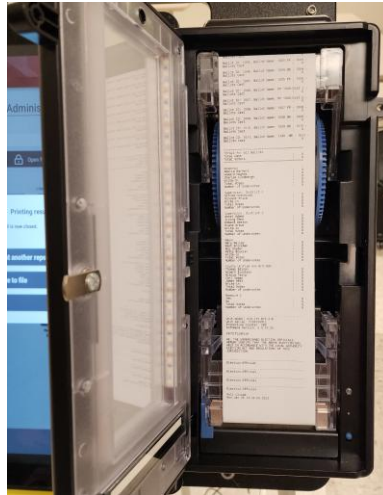
Figure 47. Opening VVPAT Printer Door to Sign Zero Report
