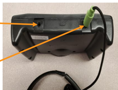
Figure 33. ATI Unit headset connection
