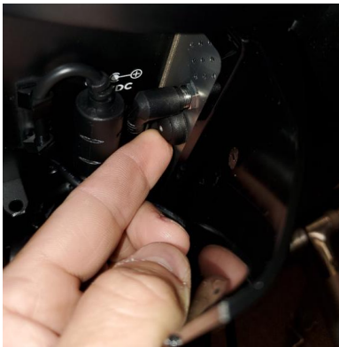
Figure 38. Press down ICX power button
