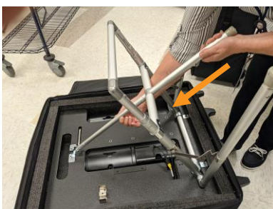
Figure 84. Collapse Center Guide Bar
