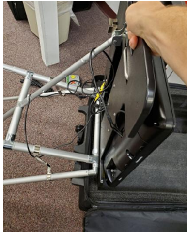
Figure 14. Check the printer attachment and roll the machine onto its base
