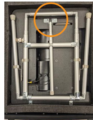
Figure 86. Legs fully collapsed
