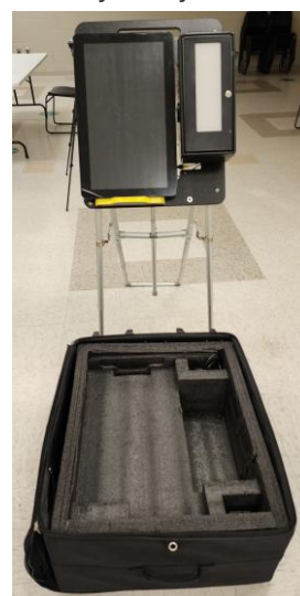
Figure 81. ICX Machine aligned 18-24" in front of the case
