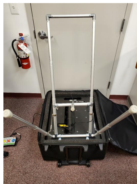
Figure 12. ICX Stand properly extended
