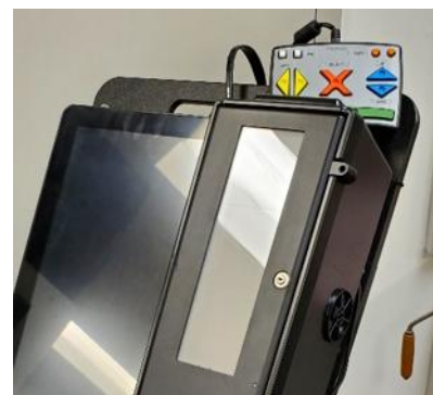
Figure 34. ICX #1 with ATI Unit
